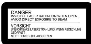
This label is located on the top of the drive unit enclosure.
