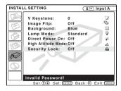
**4** Turn the main power off and disconnect the AC power cord. The security lock is set to on, then it becomes effective. The screen for entering the password is displayed when the power is turned on the next time.
