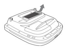
4 Remove the air filter from the 6 tabs of the air filter cover.
