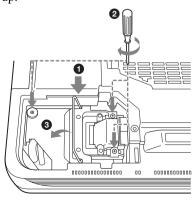
**6** Insert the new lamp all the way in until it is securely in place. Tighten the two screws. Fold down the handle.
