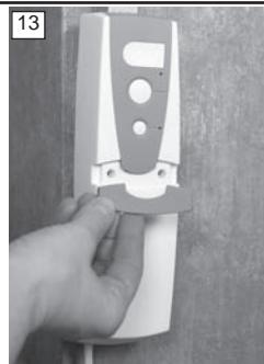
**Installation of light sensor GWLS1 (accessory):**
