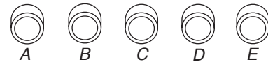
A. On/Off light button B. Blower Off button C. Blower speed minimum button D. Blower speed medium button E. Blower speed maximum button
