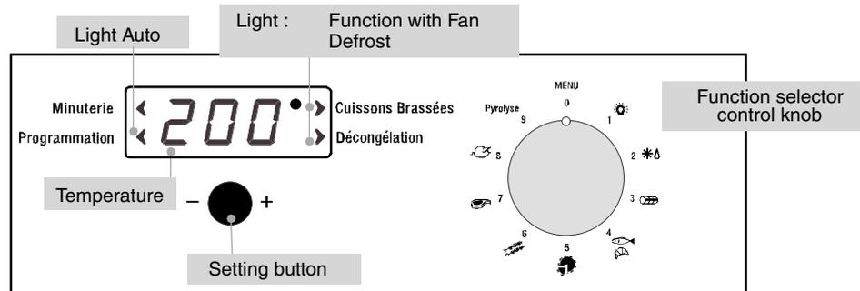
**200°** The temperature indicator “ ° ” pulsates until the pre-set temperature is not reached
