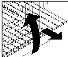
The oven features a new shelf safety system. This allows you to pull out the oven shelves when inspecting the food without danger of food spillages or shelves falling accidentally out of the oven.
