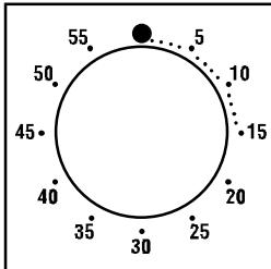
To set the cooking time, turn dial one complete revolution and then position the index to the required time. When the time has lapsed, the signal will ring for a few seconds.
