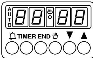
**WARNING : the first operation to carry out after the oven has been installed or following the interruption of power supply (this is recognizable the display pulsating and showing 0:00) is setting the correct time. This is achieved as follows**
