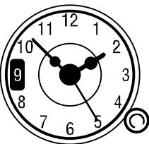
To set the time, pull the control knob and turn clockwise to position at the correct time. To set as minute minder, set the cooking time by turning clockwise the knob without pushing, until the desired time is shown at the small window on the left of the clock (max. 180 minutes). When the preset time is elapsed the alarm will ring and the oven must be switched off manually. To stop the alarm turn the knob until **X** appears in the window.
