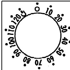
This control enables to set the desired cooking time (max. 120 min.) the oven will automatically switch off at the end of the set time.
