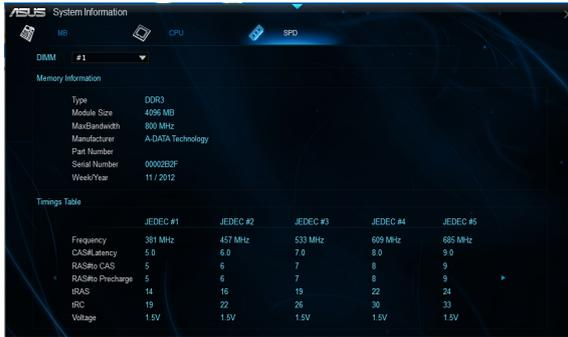
The screenshot shows the 'System Information' window with the 'SPD' tab selected. It displays memory details for DIMM #1, including type, capacity, speed, manufacturer, and part number. Below this is a 'Timings Table' with columns for JEDEC #1 through #5 and rows for various timing parameters.
