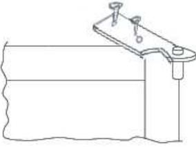
Before reassemble the hinge to the left side, reverse the direction of the hinge.
