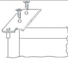
Remove the plug on the left-hand side and insert it on the right hand-side of the door.
