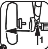
To mount the front wheels, push the wheels into the fittings until they click into place.
